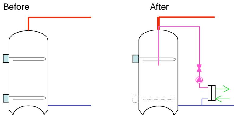
Fig 2d Details of Pipe in Pipe connection
