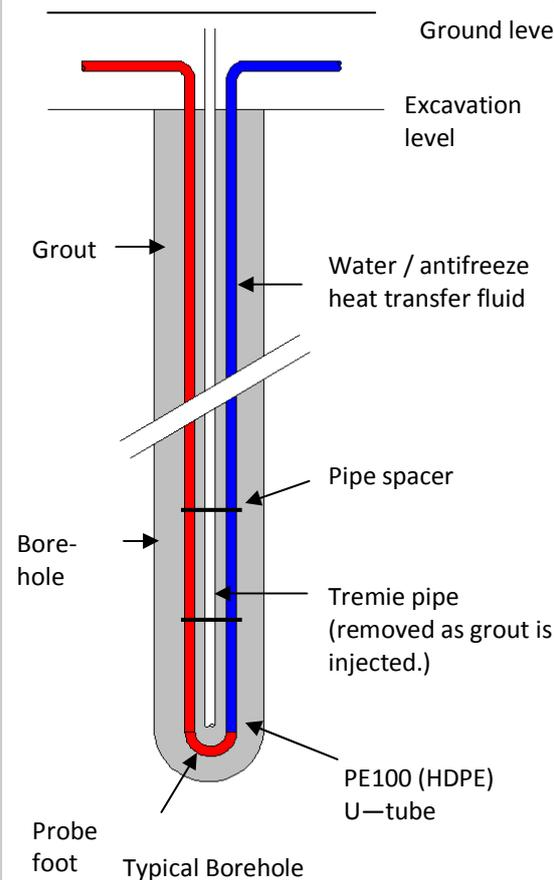
from the borehole only increases by an approximate factor of 1.25. (This is dependant on the hole and pipe diameter, distance from the next borehole, how the pipe is inserted, grouting, etc). The pipe is generally either filled with water or weighted at the end to aid with the insertion.
